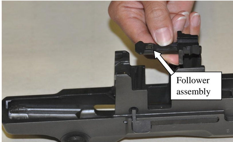
Figure 18. Follower assembly removal
